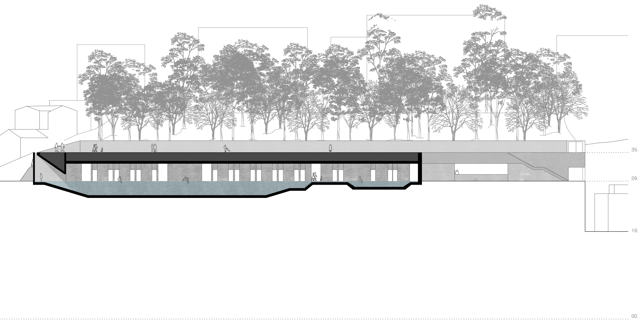
Longitudinal Section 1 through the covered swimming pool.
