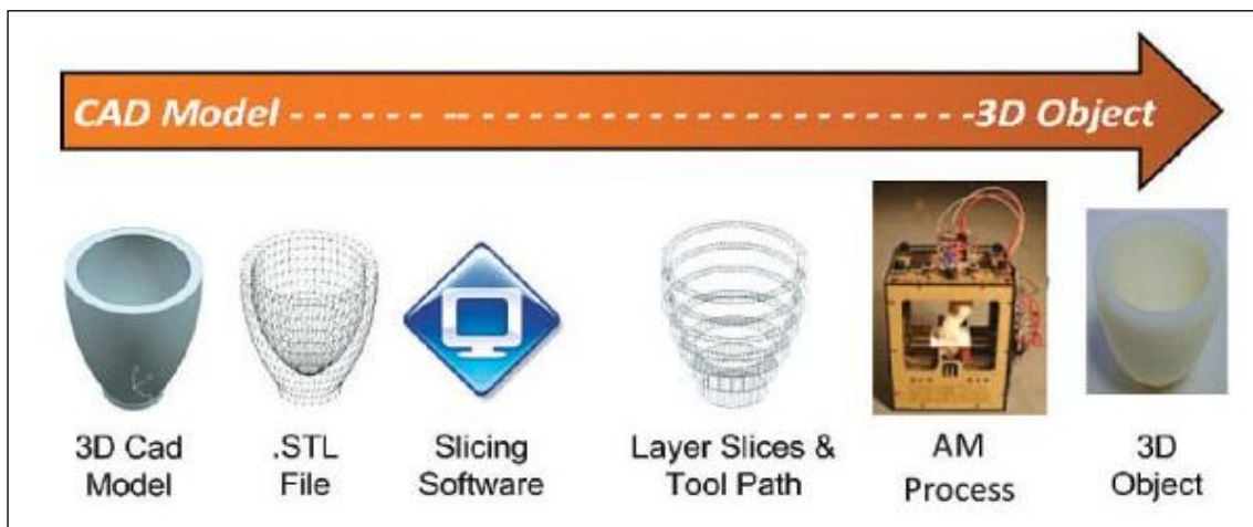
Figure 1 – Generalised steps of the 3D printing process (Campbell et al., 2011)
